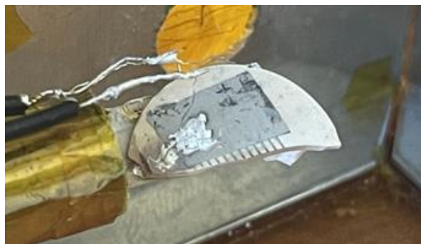
Figure S5 Image of Sample A connected to in-situ measurement setup with 5x9 mm Pt Electrode on the front side.
