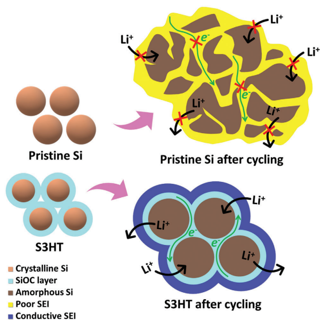
Figure 9. Schematic illustration of structure evolution of pristine Si and S3HT electrodes after charge-discharge cycling.
